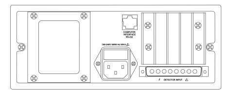
Figure 2-1. Model 35360A TRACKER Display Rear Panel
